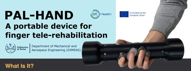
PAL-HAND is a lighweight, untethered device designed for active post-stroke finger rehabilitation. It integrates 5 pneumatic soft sensing chambers (SPSCs) to provide localized kinesthetic and vibrotactile feedback on each fingertip, enabling telerehabilitation in home or XR environments
